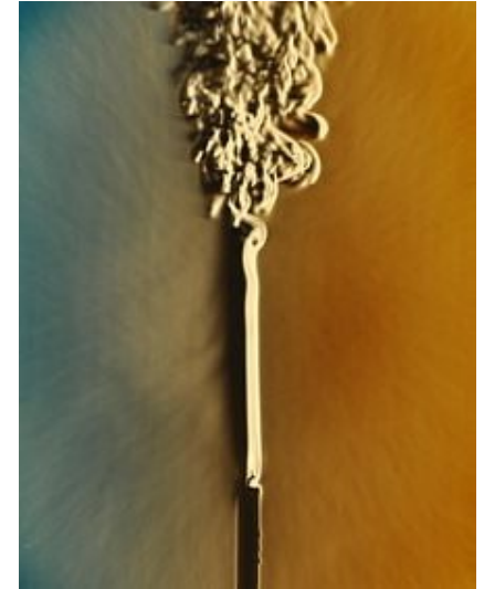
Candle plume transitions from laminar to turbulent (from https://en.wikipedia.org/wiki/Reynolds_number )
